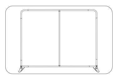
**Step 4:** Fix the base stands to the frame.
