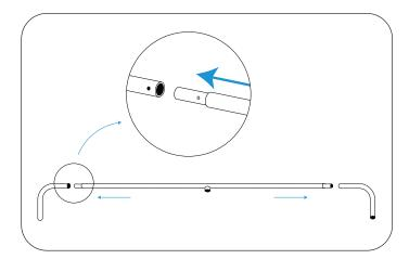
**Step 1:** Begin assembling the frame by connecting the top tubes.
