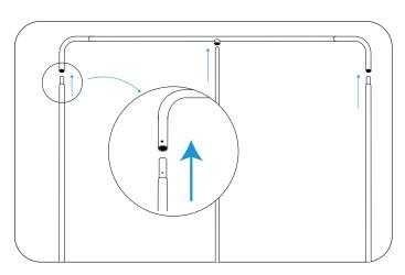
**Step 2:** Attach the vertical tubes to the top corners.
