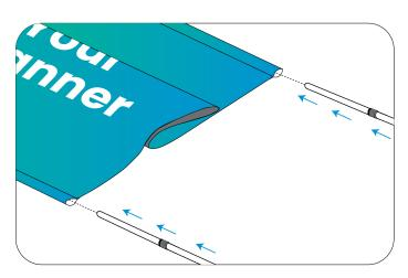
**Step 4:** Insert the horizontal poles into the pole pockets at the top and bottom of your banner.
