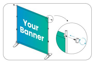
**Step 6:** Attach the top horizontal pole to the top of the vertical poles and screw it in place.
