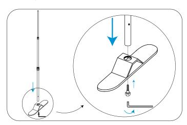
**Step 3:** Insert the vertical poles into the bases of the stand and screw them into place.
