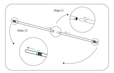
**Step 1.1:** Join the parts of the two horizontal poles.
