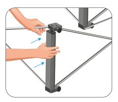
**Step 2:** Lay the structure down and install the corner supports.
