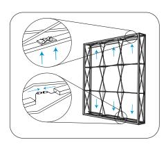
**Step 5:** Secure the LED light bars to the top and bottom of the frame and connect the wires.
