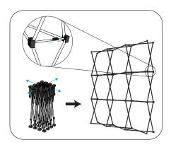
**Step 1:** Expand the display frame and lock the support arms.
