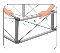
**Step 4:** Flip the frame over and install the remaining channel bars.
