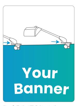
**Step 2:** Fix the LED light onto the hanger.
