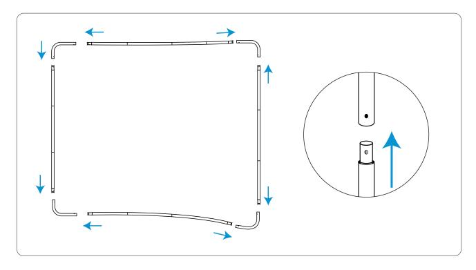
**Step 1:** Connect the numbered aluminum tubes, following the labels to quickly assemble the curved frame.
