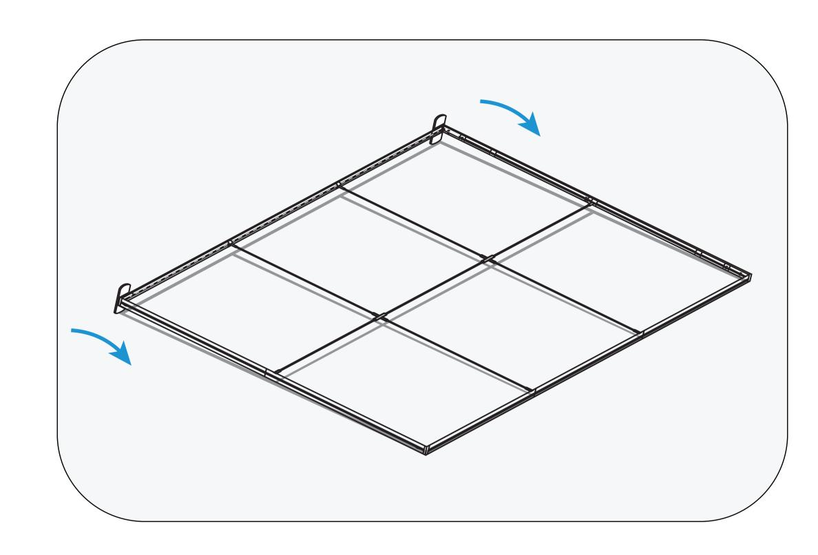
Step 3: Position Frame Face-Down: Place the assembled frame face down.
