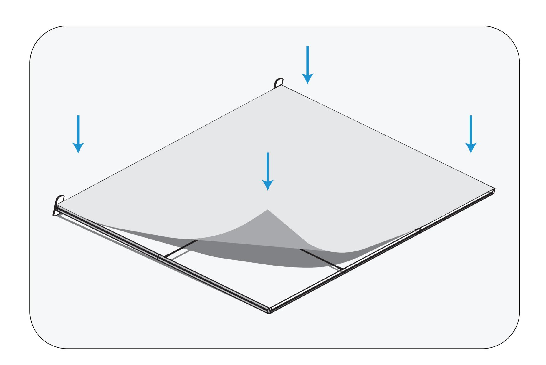
**Step 4: Install Blockout Banner:** Install the blockout banner from the back side of the frame.
