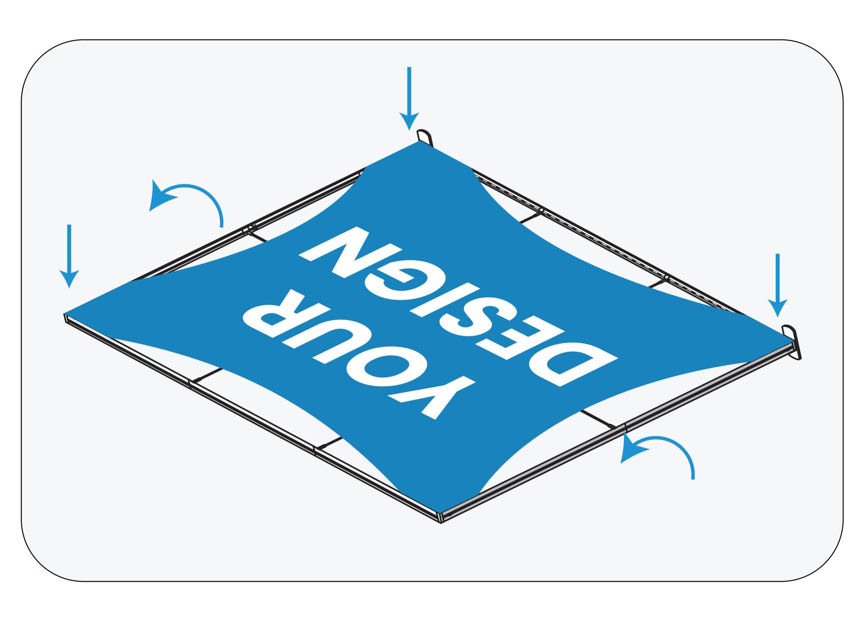
Step 5: Flip Frame Face-Up & Install SEG Graphic: Start at corners and tuck the silicone edges into the grooves.
